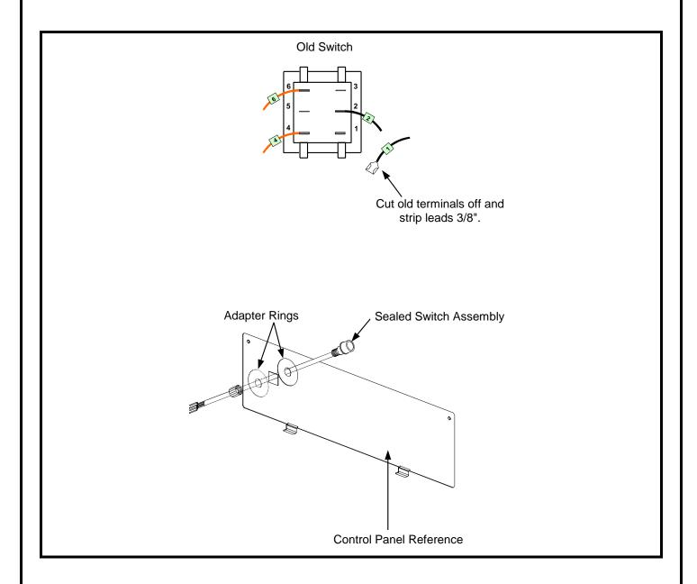
The sealed switch assembly (Part # 807-3755) is used to replace damaged or defective rocker switches on older Dean fryers. Disconnect fryer from power source. Remove the control panel to gain access to the old switch and install the sealed switch assembly as follows:
